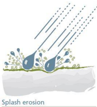
Figure 5 splash erosion occurs when individual raindrops fall on bare soil. This will usually result in rill and gully erosion and is collectively known as hillslope erosion Adapted from Saving Soil, NSW DPI.
